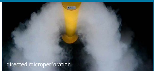
Examples of airflow patterns created through a smoke test in the PRIHODA testing center
